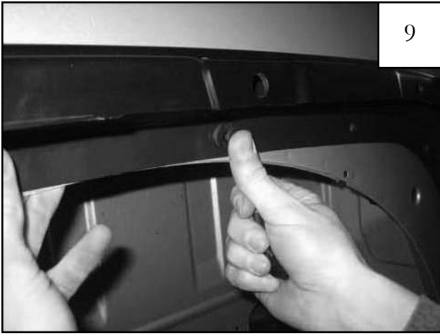
Position Inner Flare Piece on fender, aligning existing 5/16" holes in Inner Flare Piece with holes in fender. Install supplied Plastic Push Retainers (RV1-P006) (9 places).
